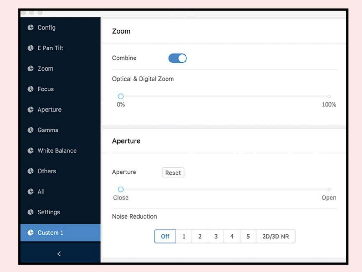
Vidtek has developed an intuitive control software and API for Sony block cameras. Our highly customizable user friendly software works with VTK-520A series and FCB-EV7520A.
